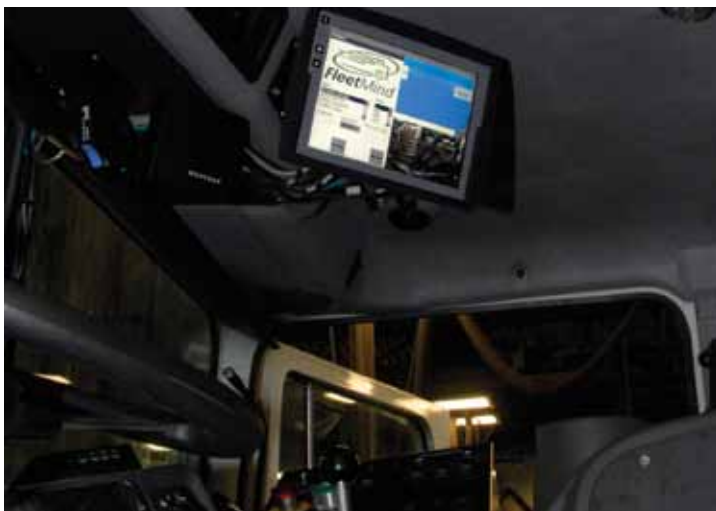
In-cab touch screen for route management and driver direction. Images courtesy of Fleetmind.
