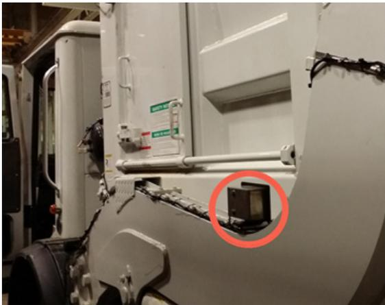
Lift Sensor/Actuator for Commercial Waste Vehicles
