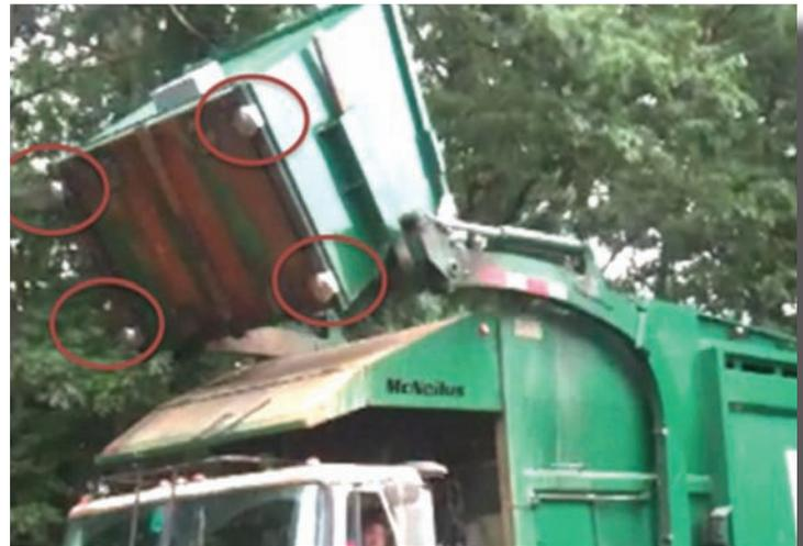
Smart trucks can now come with calibrated mobile scales that record the weight of each cart/container lifted.
