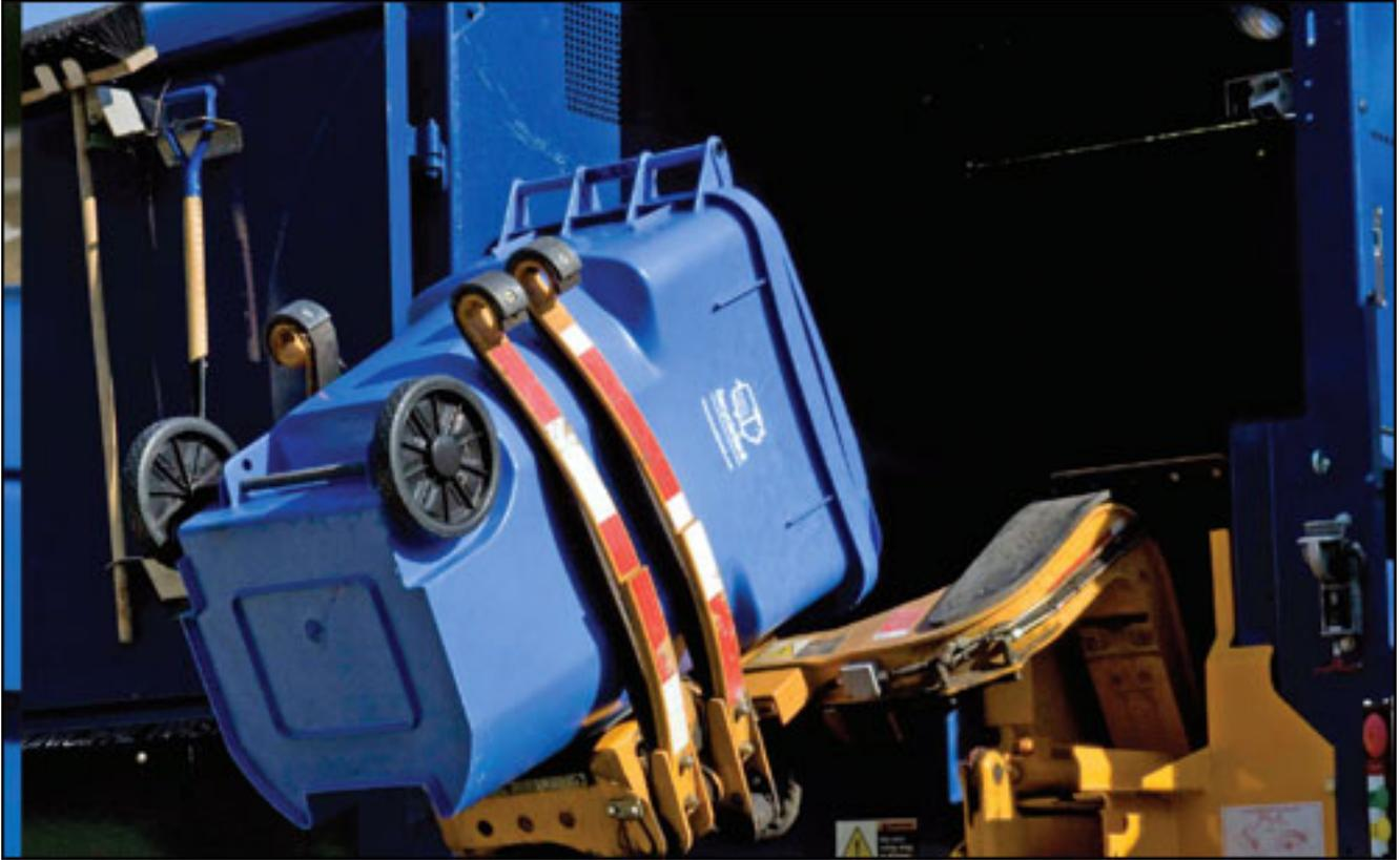
*When an RFID-tagged container is tipped into a truck equipped with an RFID reader, the reader captures the tag's identification number, associating garbage or recyclables with a householder's account. (Photo: Recyclebank)*
