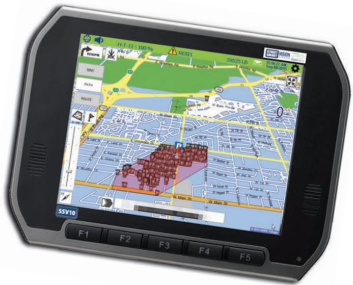
Right: Sample view of DVR monitor. In-vehicle software enables the driver to show the navigation panel in full-screen mode and view the route polygon, vehicle path and bins.
