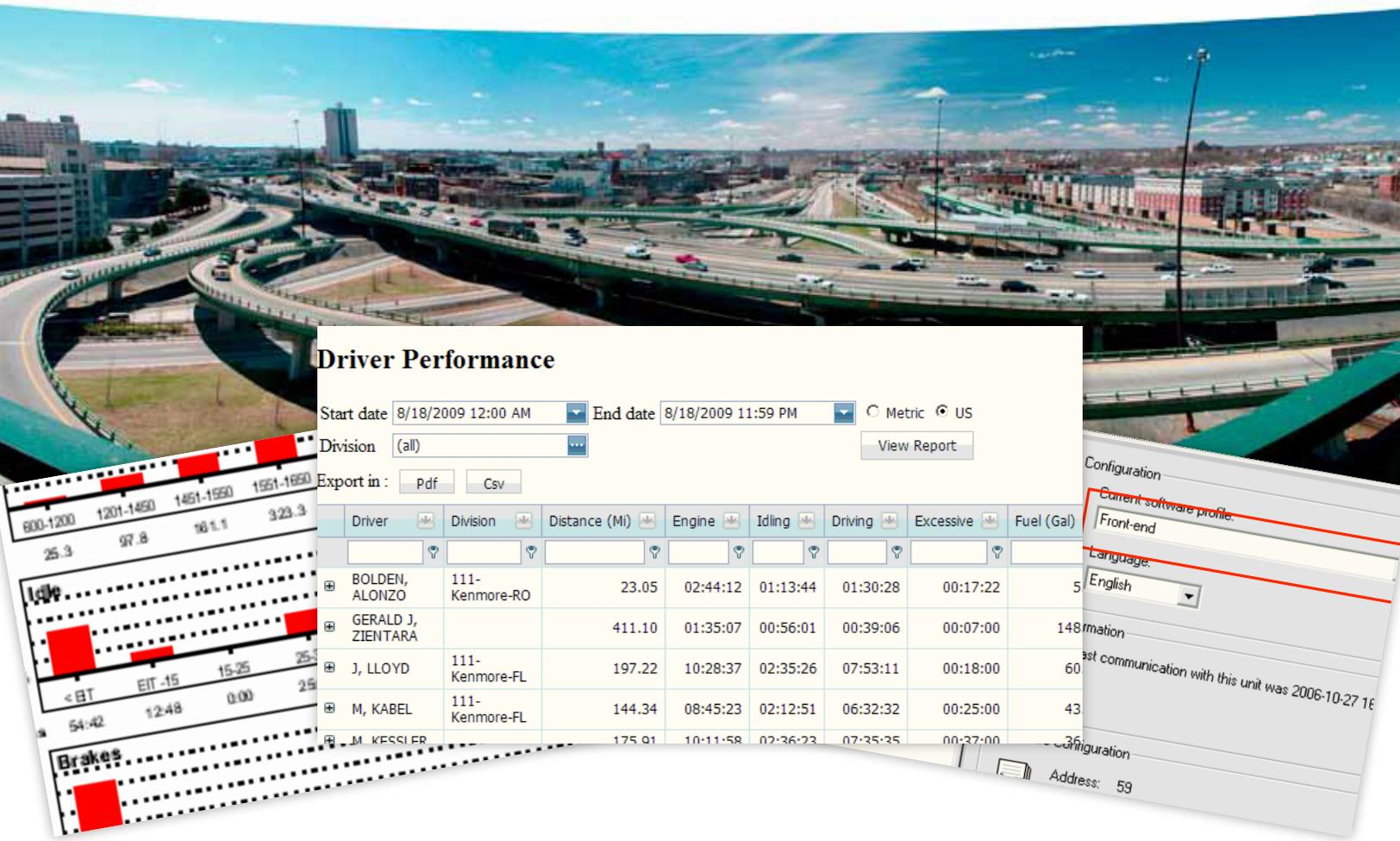
FleetMind combines its onboard computer (OBC) with mobile communications capabilities to capture and store electronic control module (ECM) and other vehicular data to provide accurate performance reporting and real-time alerts. This information is essential toward improving fleet performance and reducing costs.
